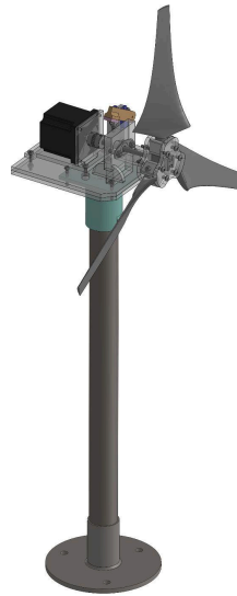
Figure 1: CAD of full turbine assembly. The main components are the rotor, nacelle, foundation, and braking system.
